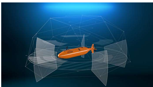
Figure 5.11 HUGIN is a free-swimming autonomous underwater vehicle (Illustration: Kongsberg Maritime).
