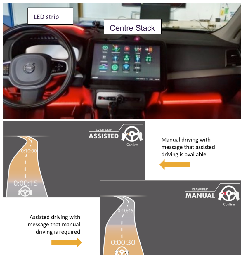
Figure 6. Top: LED strips used inside the cabin of the test vehicle to show the driving mode of the in-vehicle prototype. Bottom: HMI example shown in the centre stack of the test vehicle (adopted from Fiorentino et al., 2023).
