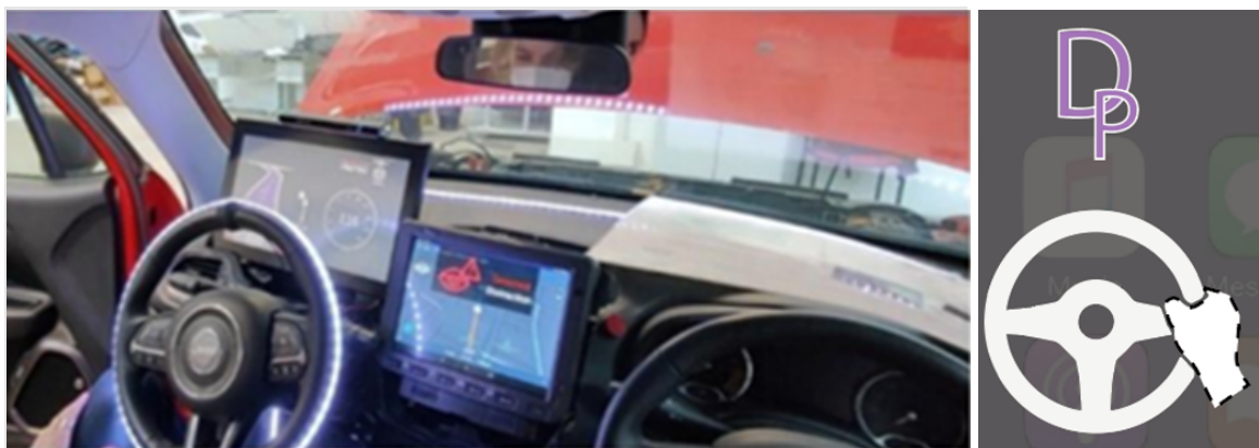
Figure 4. Left: HMI stimuli on cluster, head unit and LEDs on steering wheel. Right: Automated driving mode icon (adopted from Fiorentino et al., 2023).
