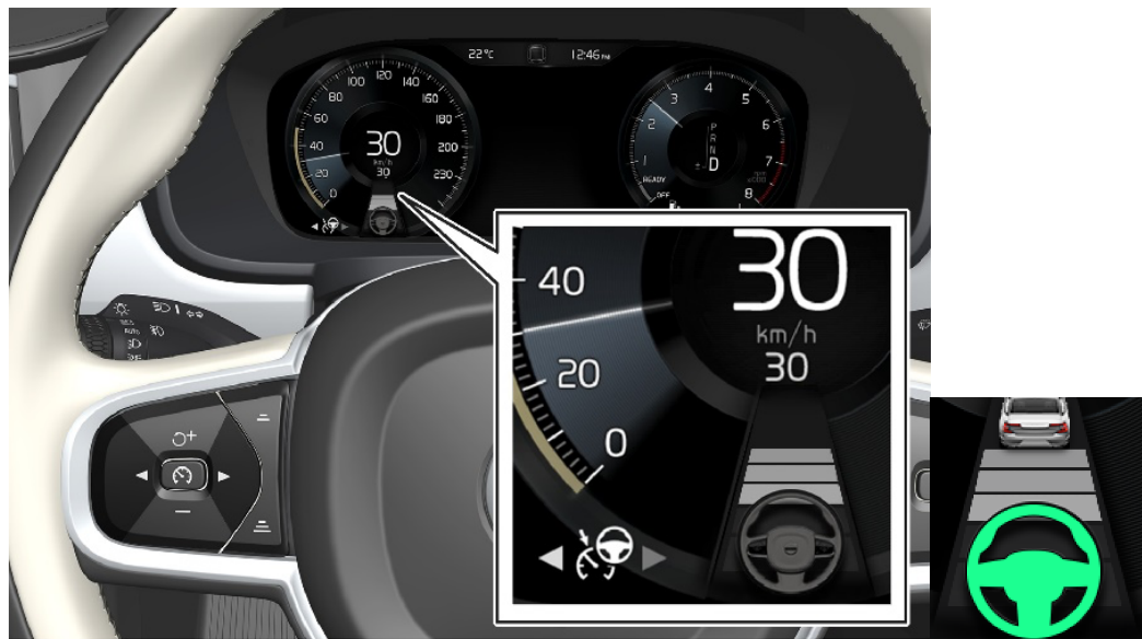
Figure 12. Pilot assist, when the steering wheel is grey the pilot assist is activated but the steering assist is not active. When the steering wheel is green the steering assist is active.
