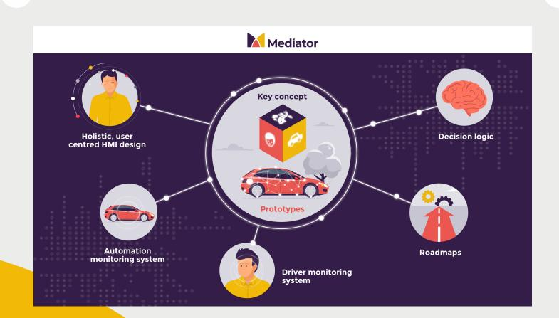
The Mediator system, as developed in the project, consists of four main modules: a driver monitoring system, an automation monitoring system, a human-machine interface and a decision making module.
