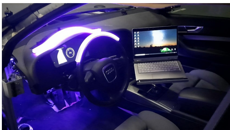
Figure 25 Hardware for controlling the three WS2812b LED strips based on Arduino Due with the PC power supply (top left), after integration under the engine hood of the driving simulator (right) and active in SB automation mode with footwell lighting and laptop for secondary tasks (bottom left)
