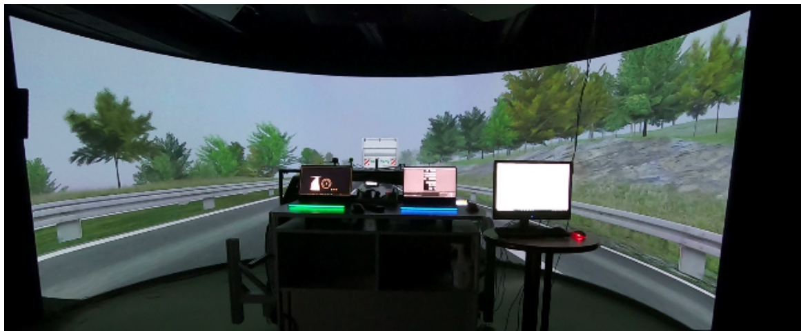
Figure 24 TUC driving simulator before adding the Mediator lab prototype (top left), full scenery during a Mediator trip with the three Mediator computers in the back (bottom) and closer look (top right) to the Mediator laptop showing the instrument cluster (green front light) and data display laptop (blue front light).
