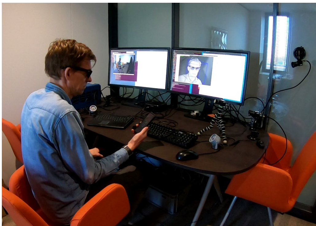
Figure 10 Lab prototype hardware set-up during a real-time cameras-based Driver State component test. In this example, the “driver” wears sunglasses, and the NIR-sensitive camera set-up supported by NIR illuminators set-up which is able to look through sunglasses is tested in conjunction with other components.
