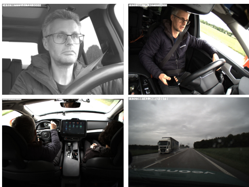
Figure 15 Example logged camera images from the four cameras installed in the T1 vehicle, replayed for Driver State oriented lab prototype tests.
