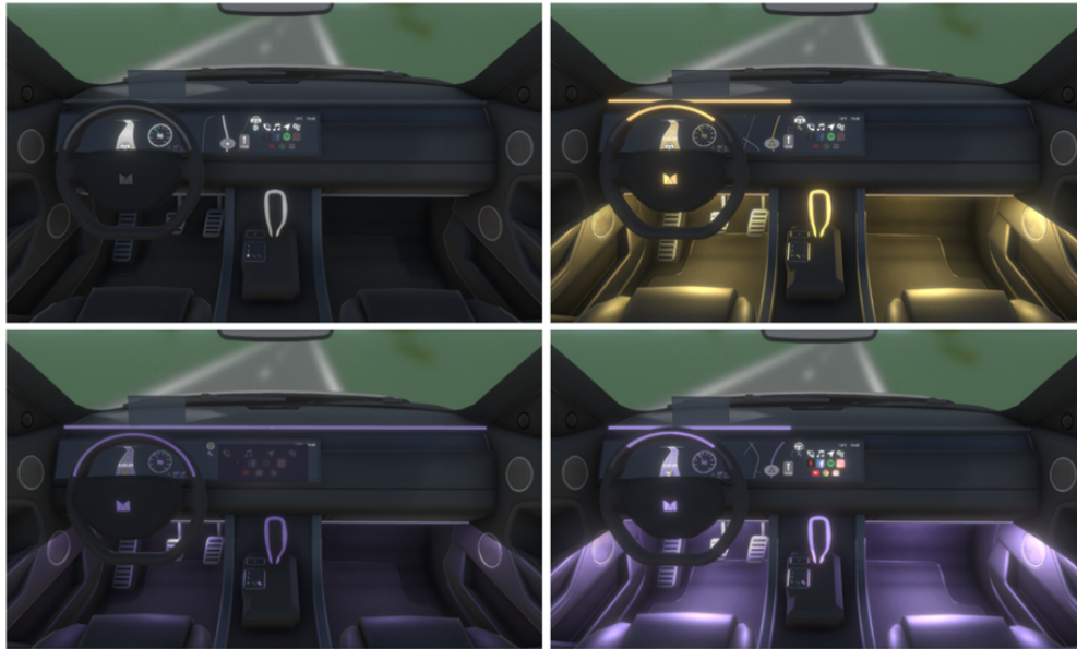
Figure 3; Mode awareness through Ambience, clockwise from top left: Manual, Assisted, Piloted (Driver standby) and Piloted dark mode (Time-to-Sleep).
