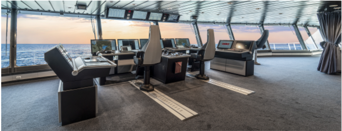
Figure 6: Colour Hybrid bridge with one workstation for manoeuvring and navigation, and one for monitoring.
